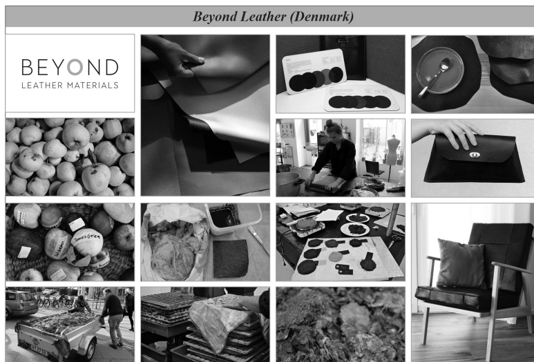
Figure 9. Compilation of images showing Beyond Leather's vegan leather biomaterial made from the residue of apple processing to produce juice and ciders, details of the manufacturing process and some of its possible applications. Source: (Facebook: Elaborated by the authors of https://www.facebook.com/BeyondLeatherMaterials ).
